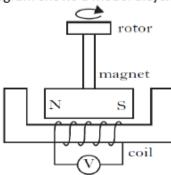
When the rotor is turned the magnet rotates, inducing a voltage in the coil.
